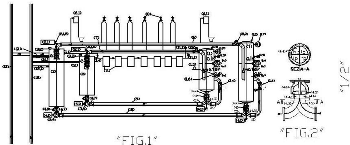
The Fig. 1 and 2 of the drawing 1/2, reported respectively the hydraulic scheme and the pump with the double separate power supply until to the impeller, the hydroelectric plant pressurized domestic, of which shows the legend:
