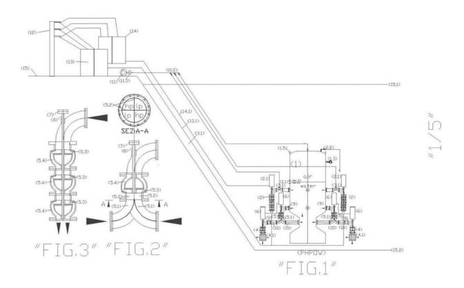
The "pressurized submerged Hydroelectric plants" in Fig.1, are resting on the seabed and produce energy with very high yields, even higher than coal, without the need to purchase fuel and release the dissolved oxygen in the water for free thanks to high tank pressure fed by an air compressor located on the shore, which also provides pressure energy, which becomes kinetic energy tath is transferred to the water and exploitable by the turbines.
