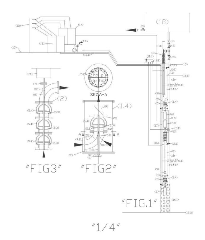
The "pressurized hydroelectric plants in" Fig.1 wells, produce energy with very high yields in the pump used as a turbine with alternator placed at the exit of the well, without the need to purchase the fuel and if the water is lifted in a tower piezometric can be distributed by gravity to subsequent
